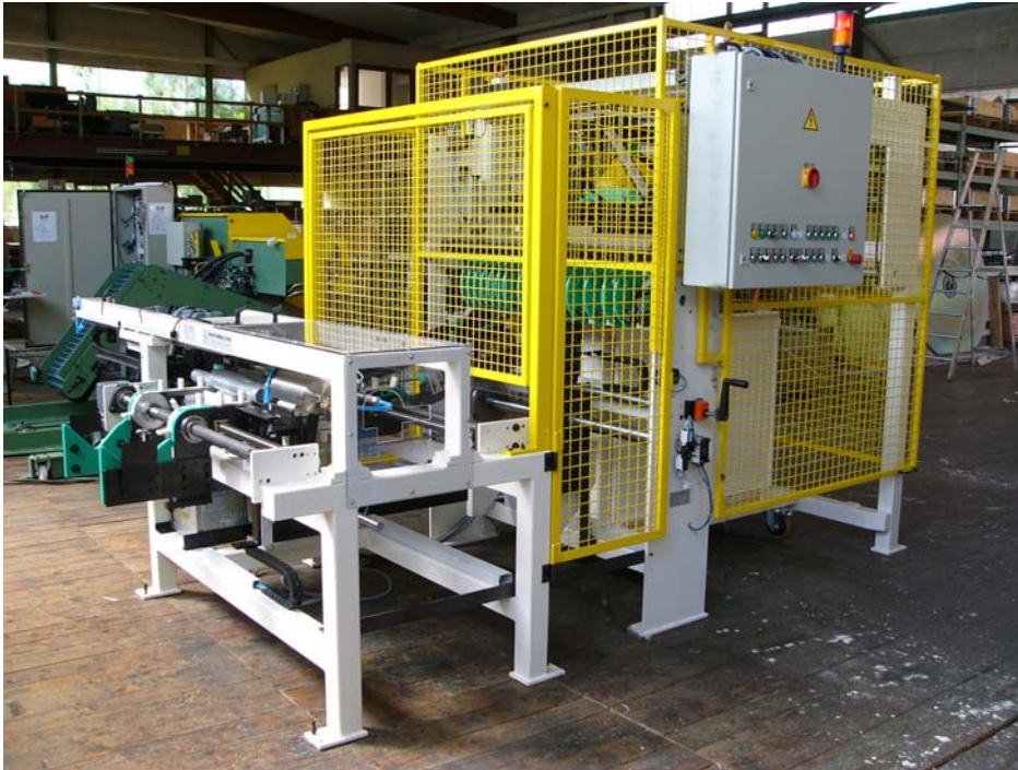
output unit with de- burring station and magazine container
