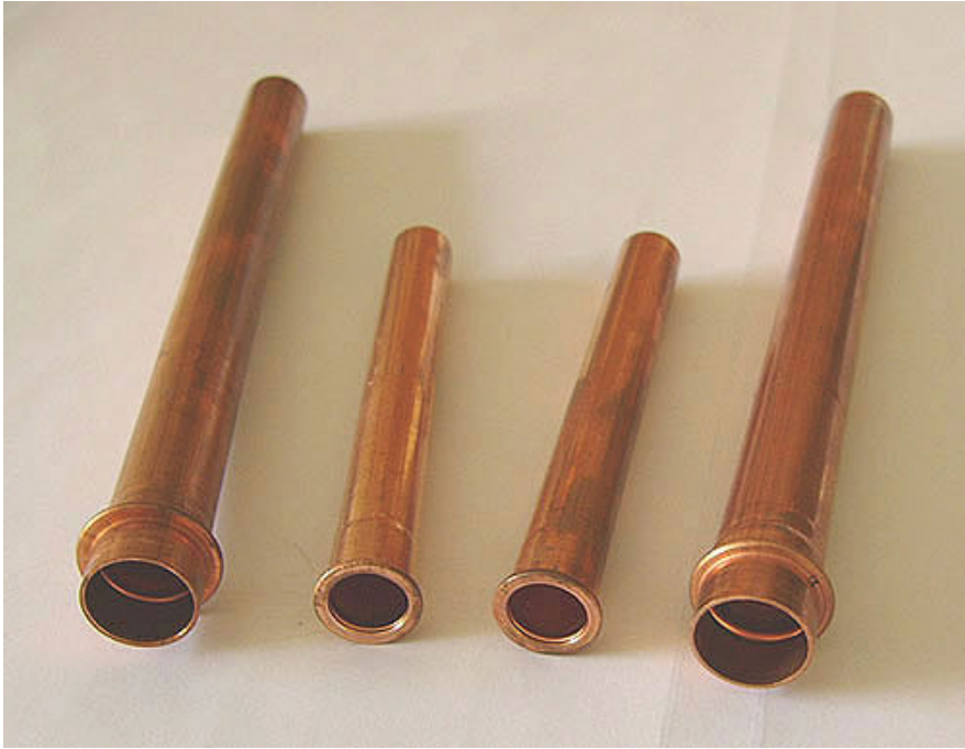
Gathered tube ends – done with an end conditioning machine
