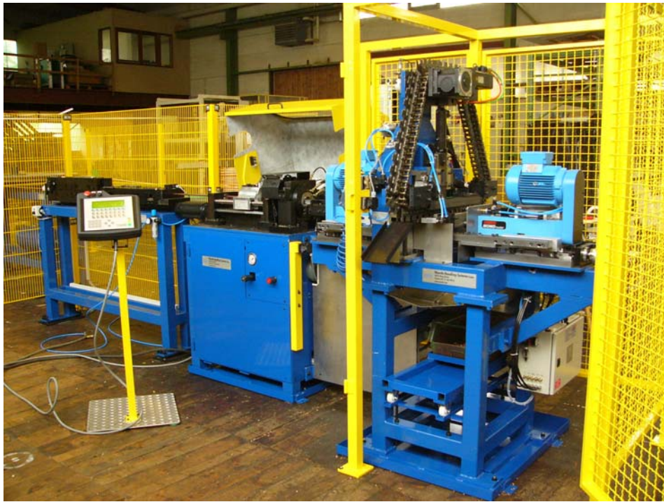
End conditioning machine interlinked with tube cutting machine RTA 35 – tube supply from a coil
