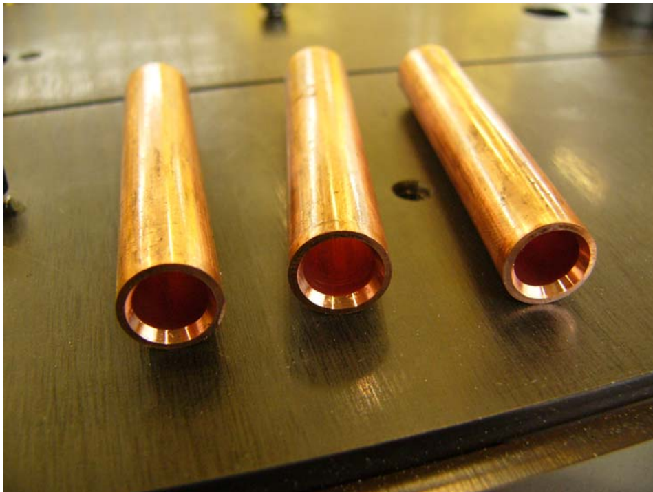
Treated tubes with strong inner chamfer
