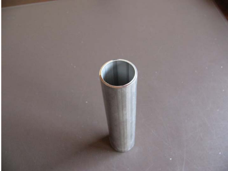
high grade steel tube, chipless cut and "torn"
