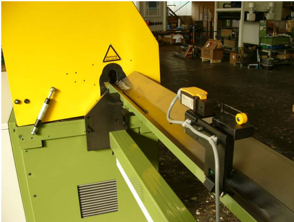
Acceptance/Taking up of cut pieces by the V-form tipping trough
