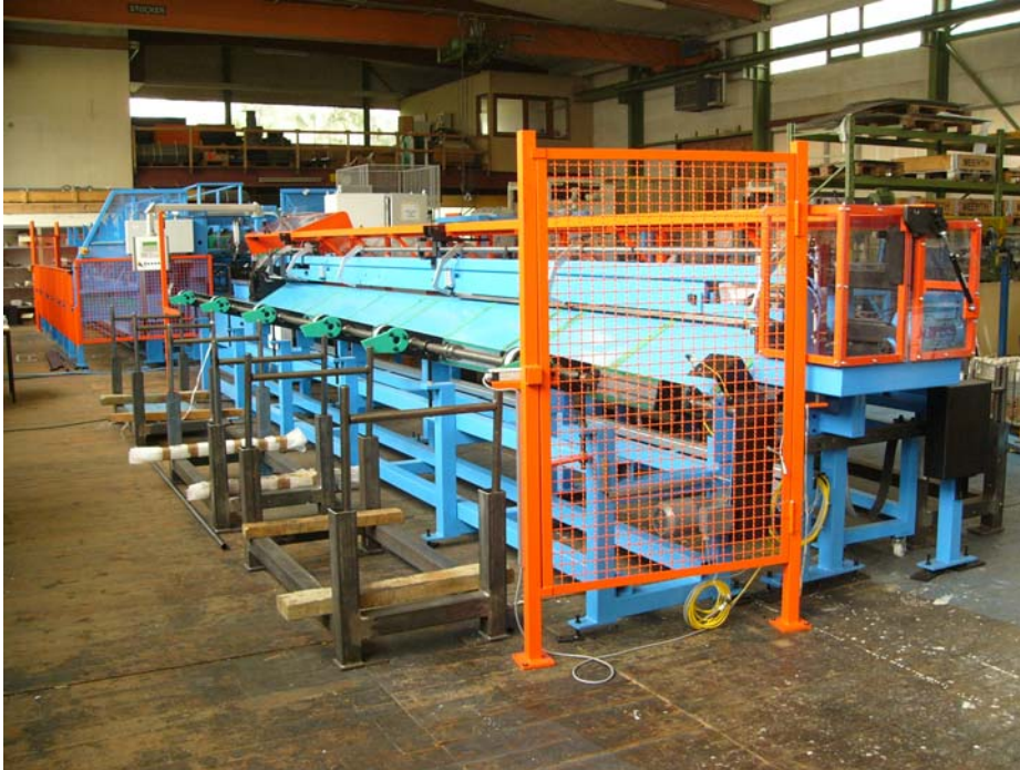
Tube cutting machine RTA 75 with 4x-bundle loader and sorting unit for long tube parts up to 5,7 m length
