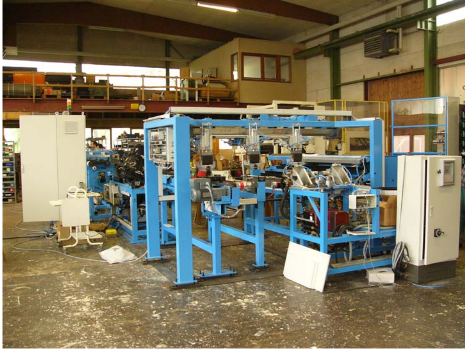
Cutting machine with grabbing system for chained working processes
