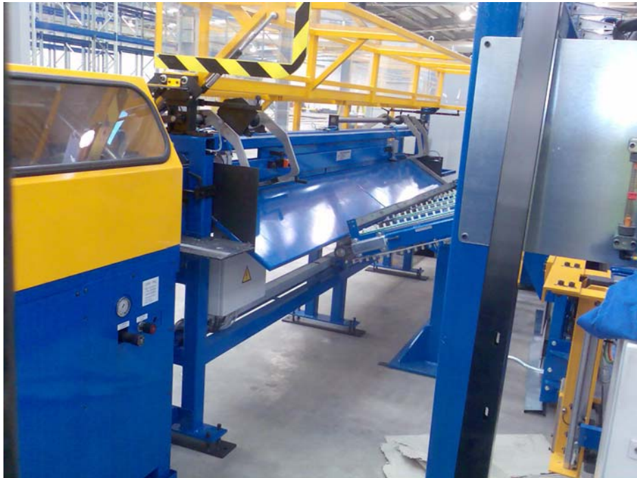
Cutting machine RTA 35 with sorting unit of different tube lengths
