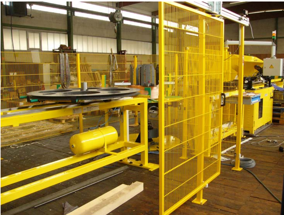
Tube coil supply to RTA 35 with uncoiler and equalizing roll
