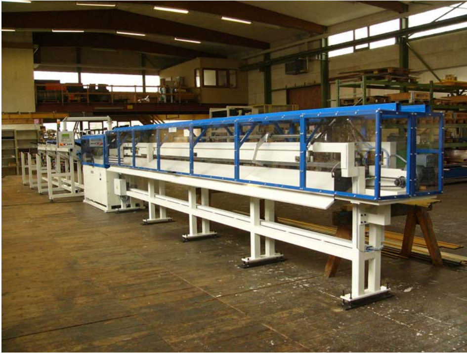
Cutting machine RTA 75 for hydraulic tubes
