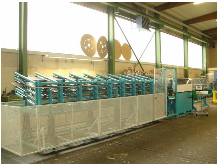
Tube cutting machine RTA 35 for small tube diameters = 4 – 12 mm
