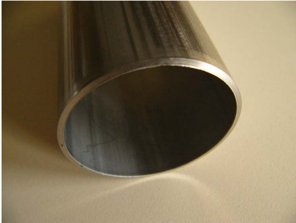
high grade steel tube, 56 x 1,5 mm, chipless cut, “torn” and “broken”
