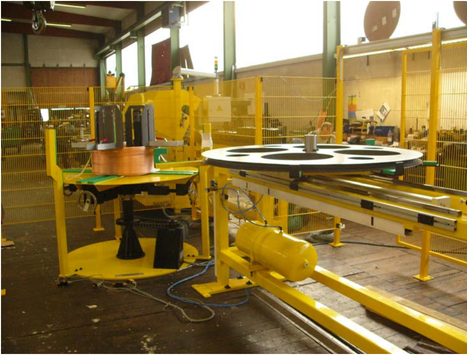
Coil-tube-supply with uncoiler and equalizing roll
