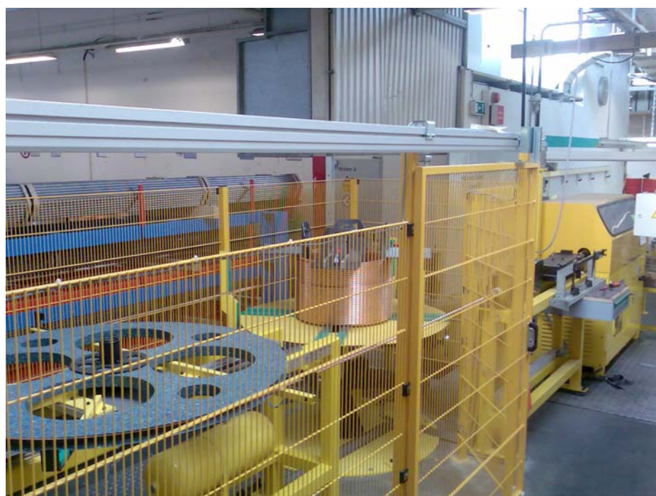
RTA 35 with tube supply from a coil
